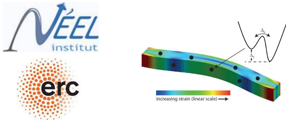
Figure: Intrinsic tunneling two level systems (TLSs) inside a glass nanomechanical resonator. The mechanical resonator will be cooled to the quantum ground state to enable measurements of the individual TLSs.
