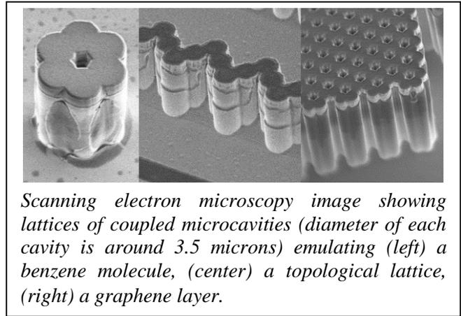
*Scanning electron microscopy image showing lattices of coupled microcavities (diameter of each cavity is around 3.5 microns) emulating (left) a benzene molecule, (center) a topological lattice, (right) a graphene layer.*
