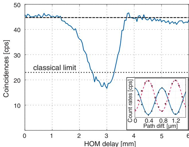
**Fig. 3. Observation of a plasmonic Hong-Ou-Mandel coalescence effect with freely propagating single SPPs on sample I.**
